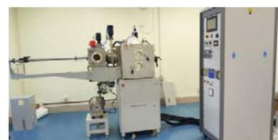
Fig 8 :RF DC Sputtering Machine
