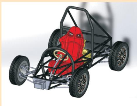
CAD design of a formulae style racing car by SUPRA, IITP
