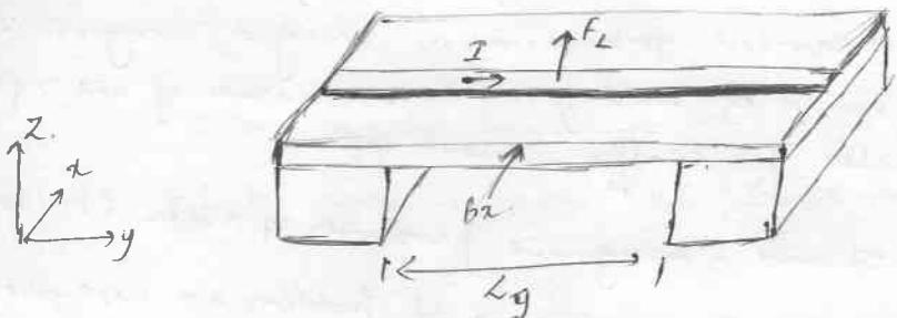
A clamped-clamped beam resonant structure. In order to excite the device a metallic loop is placed on the clamped-clamped beam surface where an excitation current ( $I_x \approx \sqrt{2} I_{\text{rms}} \sin(\omega t)$ ) flows inside it with a frequency equal to the resonant frequency of the beam. How to determine resonant frequency? → either by analytical models and simulation tools and it depends on the elastic modulus, density, deflection and geometrical features of the resonant structure.
