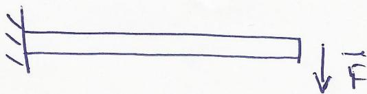
Consider the case of a cantilever beam acted upon by an external force  $F$  at one end.
