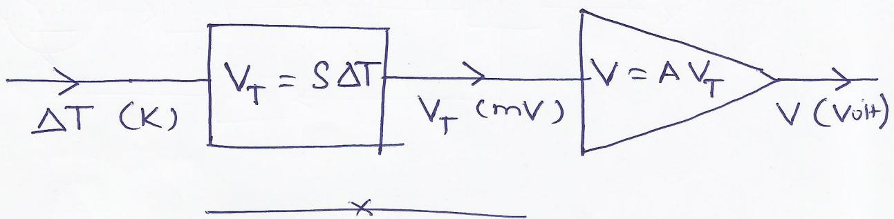
Open loop : measurement system. → Measure a variable
