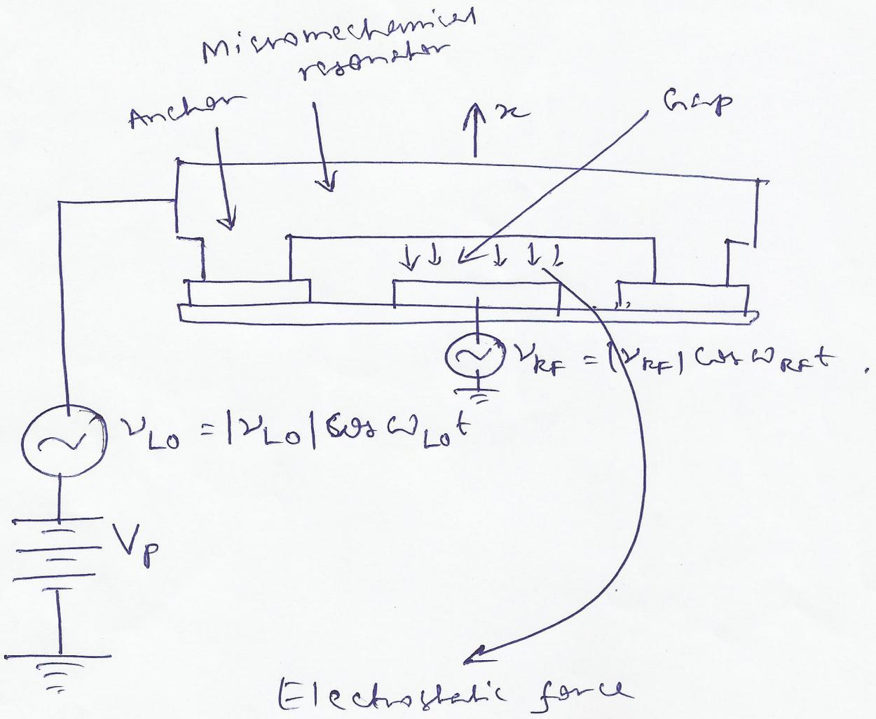
$$F_i = -\frac{\partial U}{\partial x} = -\frac{\partial}{\partial x} \left( \frac{1}{2} C_{gap} V_{gap}^2 \right)$$
