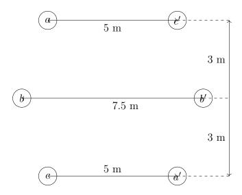
The diameter of each conductor is 15 mm.
