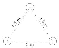
2. Determine the inductance per km of a 3-phase transmission line having conductors per phase and arranged as shown here.
